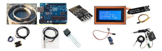
Figure 1: Double Ring Infiltrometer & Sensors
