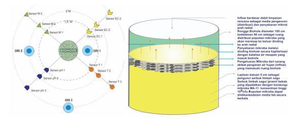
Figure 2. Distributiom Sensor Position & Biohole Structure
