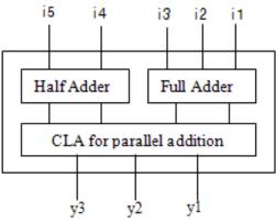
Fig.2. Block diagram of a 5-3 Compressor
