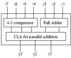
Fig.4. Block diagram of a 7-3 Compressor
