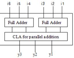
Fig.3. Block diagram of a 6-3 Compressor
