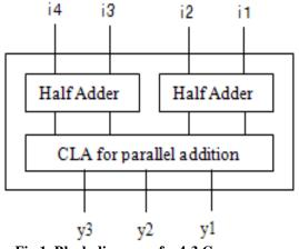
Fig.1. Block diagram of a 4-3 Compressor
