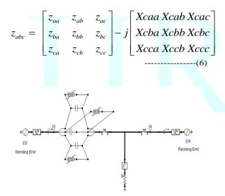
Fig.6. ATP model of the compensated transmission line.
