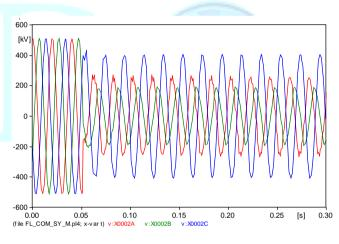
Fig.8. Fault occurred in the compensated transmission line.
