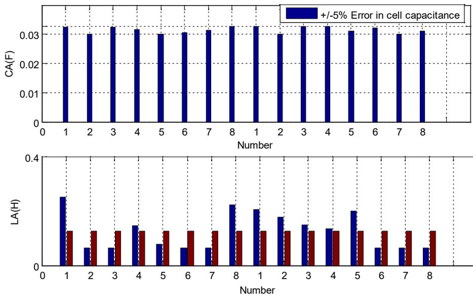
Fig.-11 Cell inductances and capacitance for configuration of two PFNs in parallel for compensating droop.
