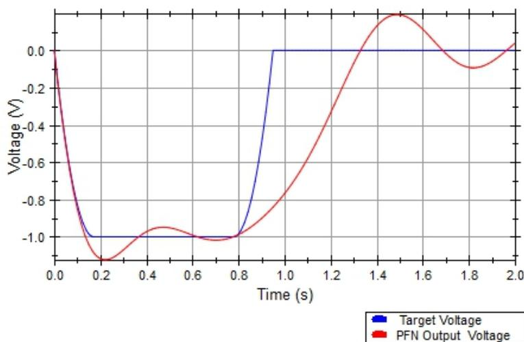
Fig. 13 The response of the PFN calculated using Green's Function and the target pulse
