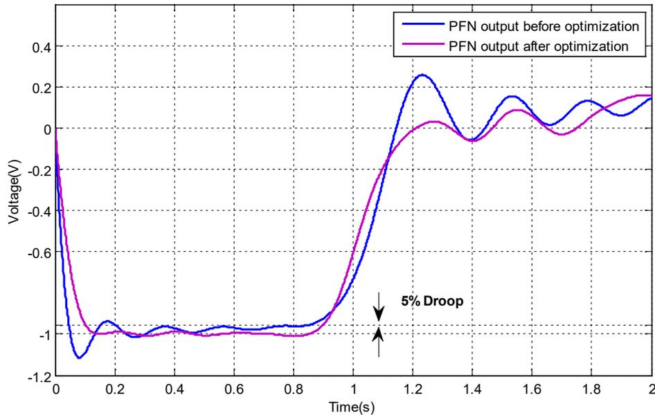
Fig.-10 Output waveform before and after optimization for configuration of two PFNs in parallel for compensating droop.
