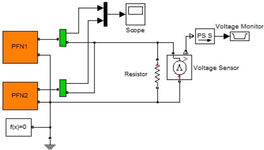
Fig. 6 Simulink Model for 2 PFN Models in Parallel
