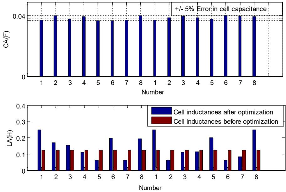
Fig. 8 Cell inductances and capacitances before and after optimization for configuration with two PFNs in parallel.
