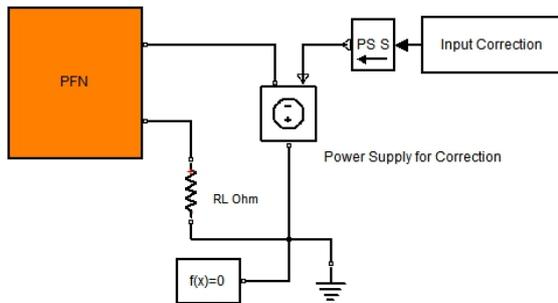
Fig. 15 Simulink Model used for validation
