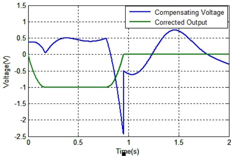
Fig.14 Compensating voltage and the output of PFN after correction.
