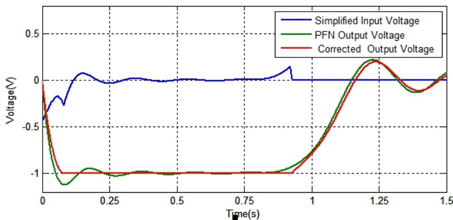
Fig. 16 PFN Output voltage of 8 cells along with the simplified compensating voltage and the corrected-out voltage.
