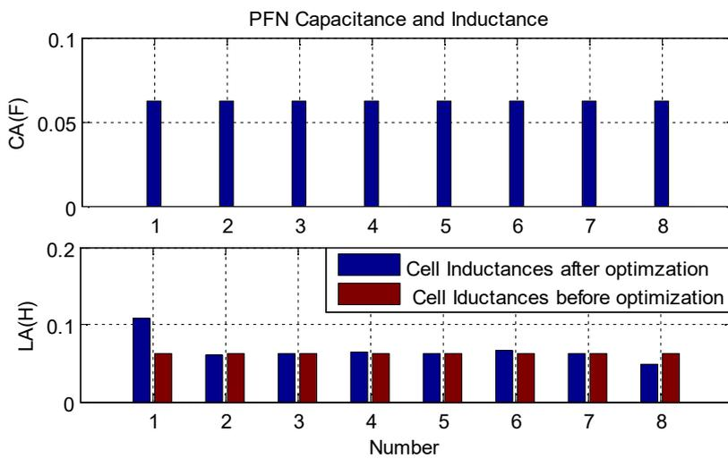
Fig. 5. Cell inductances and capacitances before and after optimization for configuration with single PFN.
