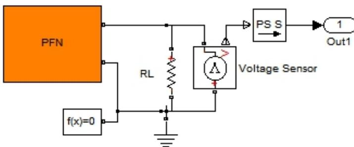
Fig. 3. Simulink Model for Single PFN with 8 cells
