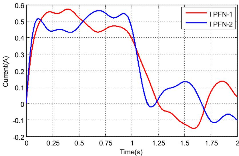
Fig. 9 Output currents from PFN-1 and PFN-2 after optimization for configuration with two PFNs in parallel.
