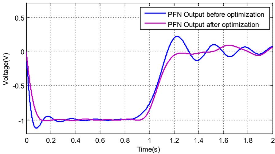
Fig. 7 Output waveforms before and after optimization for configuration with two PFNs in parallel
