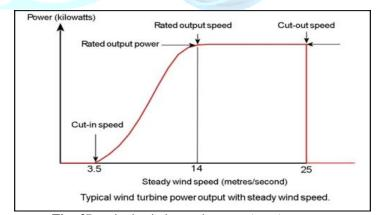
Fig-:3Required wind speed rotate (vawt)
