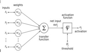
Fig.3 non-linear model of Artificial Neuron
