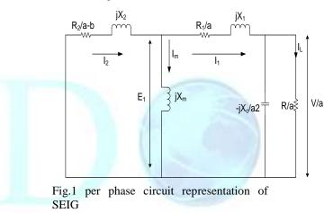
In this circuit, all the parameters are thought to be independent of immersion besides polarizing reactance. Examination of equal circuit brings about the accompanying mathematical statements for the relentless state operation.
