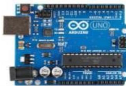
Fig. 4 Arduino Microcontroller
