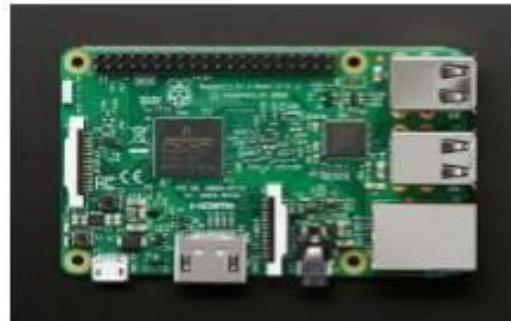
Fig. 2 Raspberry Pi 3 Model B+
