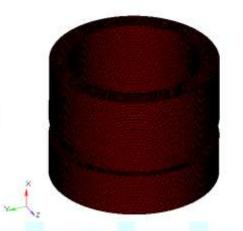
Fig-5.4: Meshed model of Bearing cup
