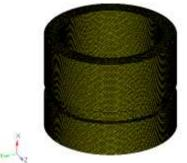
Fig-5.3: 2D Meshing of Bearing cup
