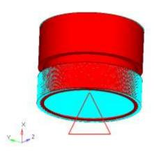
Fig-5.6: Boundary conditions applied on the bearing cup
