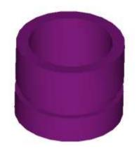
Fig-5.1 Pro-E Model of Bearing Cup
