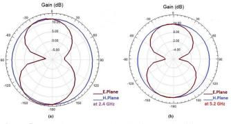
Figure 5. Radiation pattern at double frequencies (a) 2.4 GHz (b) 5.2 GHz
