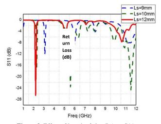
**Figure 3.** Effect of length of slot (Ls) on S11  $W_f$  is the horizontal part of the feeding element, and the S11 is changing with  $W_f$  as given in Figure 4. As  $W_f$  increases the resonant. frequency of. 2.4 GHz band decreases with the increase of  $W_f$  the resonant frequency of the high frequency band does not change. The high frequency band's bandwidth is decreased with the increase in  $W_f$ .
