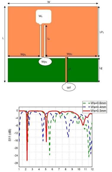
operating frequencies can be achieved as 4 dB Patch of antenna is a rectangular element whose side length is 25 mm. Appropriate gain of the antenna is ensured by reducing the volume of antenna, Number of parameters are used to measure the whole performance of an antenna. These are discussed one by one in detail along with a different parameter effects on the result.
