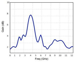
Figure 7. Proposed dual band antenna gain
