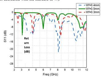
Figure 4. Effect of width of feeding line on reflection coefficient
