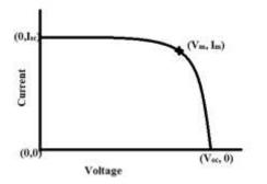
Fig 2: V-I characteristics of solar cell
