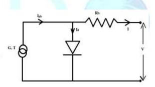
Fig 1: Equivalent circuit of solar cell
