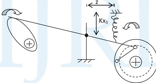
Figure 4: Cam has taken load and extending spring
