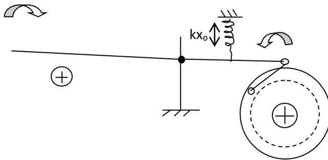
Figure 6: Cam slides off the lever, forcing the spring to return to suddenly to original  $X_0$  from extended  $X_2$
