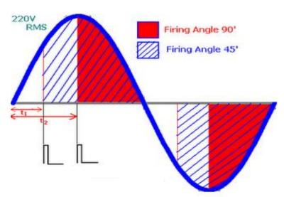
Fig.3 Representation of firing Angle of TRIAC
