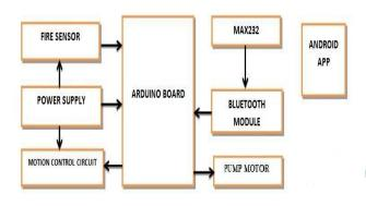
ATMEGA328P description is as follows: Each of the 14 digital pins on the Uno can be used as an input or output, using pinMode(), digitalWrite(), and digitalRead() functions. They operate at 5 volts. Each pin can provide or receive 20 mA as recommended operating condition and has an internal pull-up resistor (disconnected by default) of 20-50k ohm. A maximum of 40mA is the value that must not be exceeded on any I/O pin to avoid permanent damage to the microcontroller.
