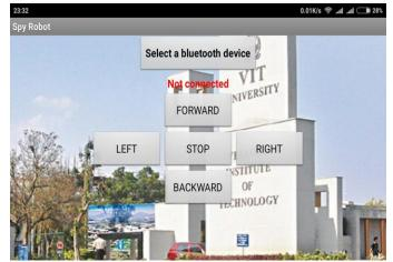
Here, different control options like forward, left, right, backward and stop are assigned from different number keys available in IOP application by default. We can connect any Bluetooth device which is compatible, The flow of control signals and its operation upon the hardware is given in the following section.
