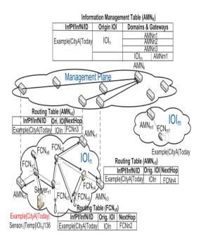
FIGURE 4. Information registration procedure in ANBR.
