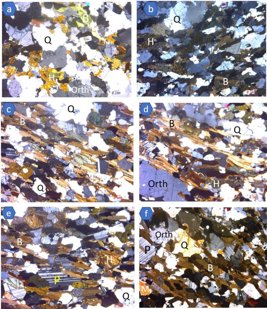
**Fig. 4: Photomicrograph of medium-grained migmatite (a-b) from Idanre area in transmitted light (cpl) showing the constituent minerals; banded-gneiss of Ita-Ogbolu (c-d); and Ado-Ekiti granite-gneiss (e-f) showing quartz grains are isolated, feldspar shows faint twinning, biotite plates are aligned and stretched in diagonal direction while opaque occur in traces. Q (quartz), B (biotite), P (plagioclase), H (hornblende), M (muscovite), Orth (orthoclase).**
