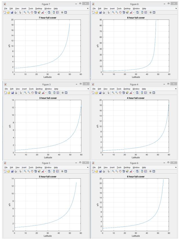
Figure 13. Graphical representation of variation of x/h ratio for different latitudes and different hours (1 to 8 hours) of full coverage.
