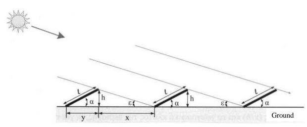
Figure 11. The geometry for the placement of consecutive PV modules of rows, on horizontal ground facing south.
