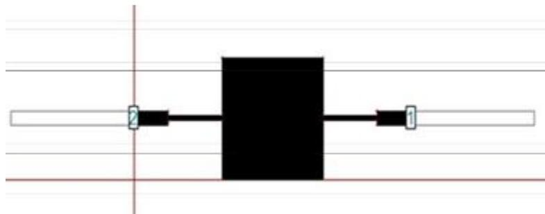
Fig.2, Layout of a 3-pole stepped impedance microstrip lowpass filter on a substrate with  $\epsilon_r = 4.4$ ,  $h = 1.5$  mm at 2.5 GHz frequency
