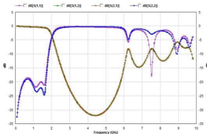
Figure 5. Full-Wave EM Simulated Performance of the Stepped Impedance Low Pass Filter for sixth order
