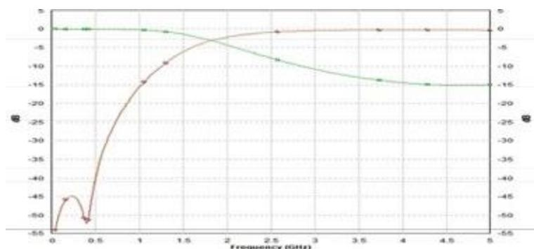
Figure 4. Full-Wave EM Simulated Performance of the Stepped Impedance Low Pass Filter for third order
