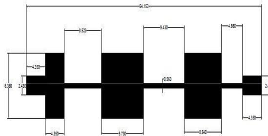
Fig.3, Layout of a 6-pole stepped impedance microstrip lowpass filter on a substrate with  $\epsilon_r=4.4$ ,  $h=1.5$ mm at 2.5GHz frequency
