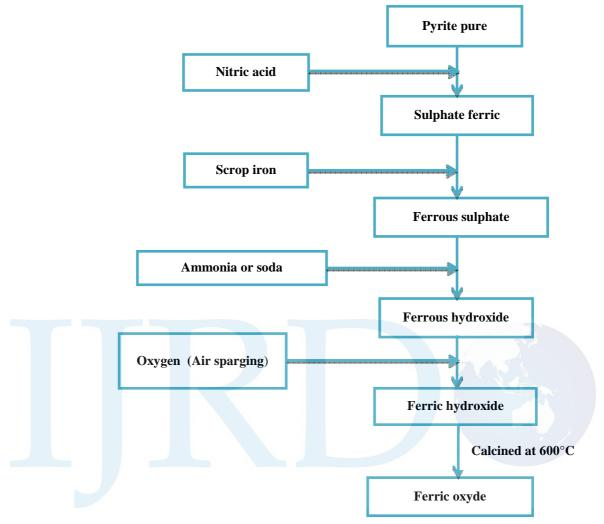
Figure 4 : Diagram of the process of synthesis of the iron oxide
