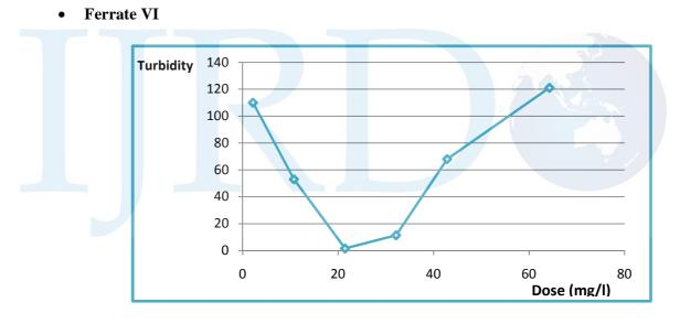
Figure 15 : Curve of determination of the optimum dose of the VI ferrate
