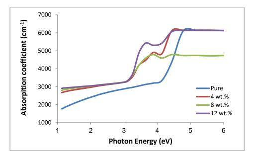
**Figure 3:** The absorption coefficient versus photon energy for (PMMA-PS-TiO<sub>2</sub>) nanocomposites
