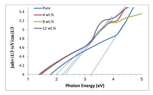
Figure (5):The plot of  $(\alpha h \upsilon)^{1/3}$  with photon energy for (PMMA-PS-TiO2) nanocomposites
