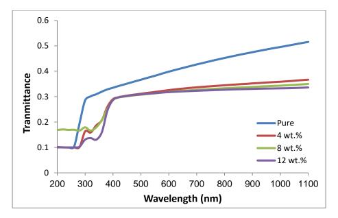
Figure (1): The transmittance versus wavelength for (PMMA-PS-TiO<sub>2</sub>) nanocomposites.
