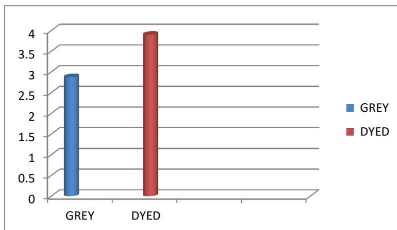
From the above table II and figure II , it was found that the abrasion resistance of dyed soya material has been increased than grey material
