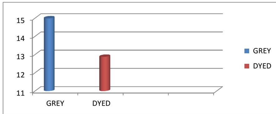
From the above table VI and figure VI, it was found that the weft shrinkage of dyed soya material has been decreased than grey material
