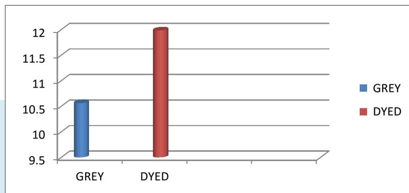
From the above table V and figure V, it was found that the warp shrinkage of dyed soya material has been increased than grey material
